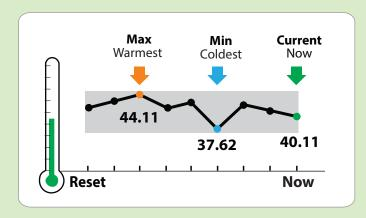
This graph shows how temperatures fluctuate during the day. Checking the CURRENT temperature is not enough. MIN and MAX temperatures are needed to catch out-of-range temperatures between now and the last time the device was reset.
